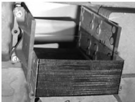
FIGURE 11 A silicon pore optics produced by stacking ribbed silicon plates. The pore size is approximately 1 \times 1 \text{ mm}^2 , the width of the stack is 68 mm.
