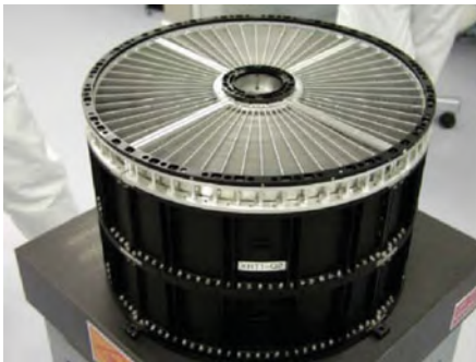
FIGURE 47.4 The segmented foil mirrors aboard the SUZAKU spacecraft. (a) A complete mirror module and (b) a single aluminum foil reflector coated with gold.
