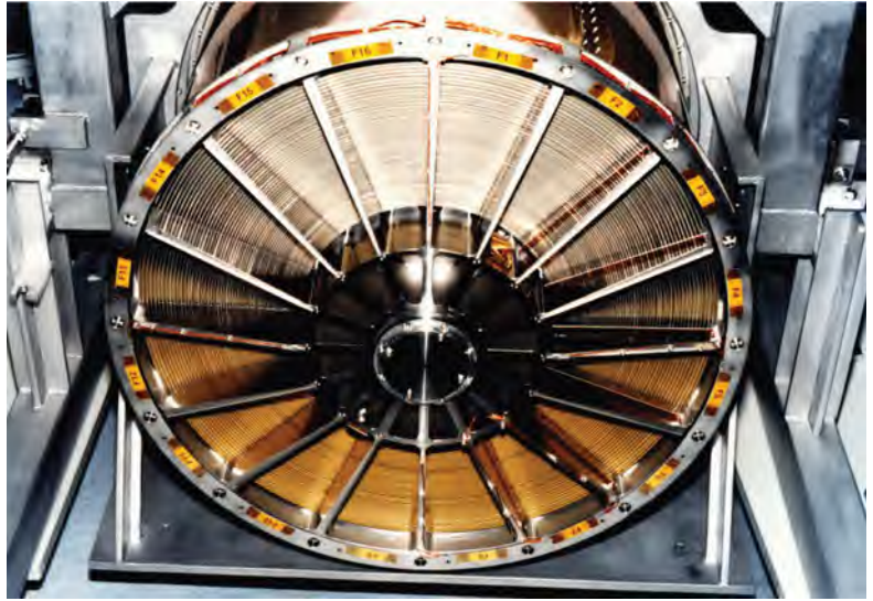
FIGURE 47.3 An x-ray optics module for the XMM observatory. Fifty-eight electroformed nickel Wolter I optics are nested to increase the effective x-ray collecting area.
