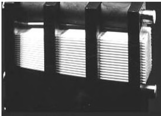
FIGURE 3 Multifiber collimating lens constructed from over a thousand individual polycapillary fibers strung through a metal grid. The lens is 10 cm long with an output of 20 \times 20 mm. The fibers are parallel at the output end (shown) and at the input end point to a common focal spot.
