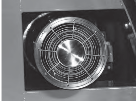
FIGURE 6 An x-ray optic module with 12 Wolter-I nested mirrors.
